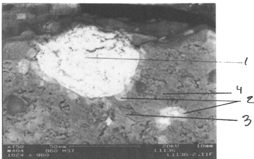
Figure 13. A Zr-containing particle from LSHS feed (4°C/min, 860°C) (SEM); 1-Zirconium silicate, 2-Sodium zirconium silicate, 3- Matrix, 4- Carnegieite.
